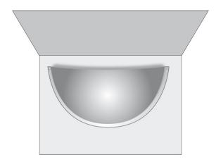
3. When installation is complete, totally remove the protective film from the face.
